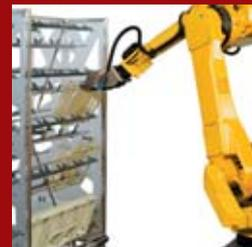
**Ares:** the most reliable, flexible semi-automated cage-handling system for medium-small laboratory animal facilities housing valuable rodents.
